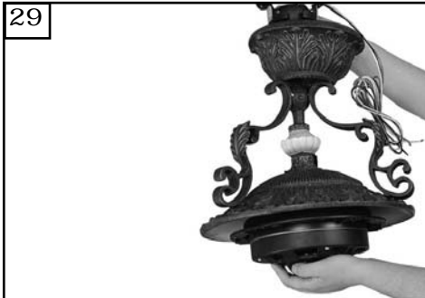
29 Raise fan with downrod assembled to the ceiling bracket and hang fan assembly. Be sure to rotate the downrod ball so that the notch in the bracket engages the slot in the ball.
